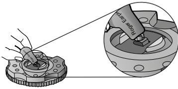
Then fit a new filter and check that the filter is properly in place.
